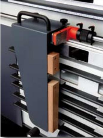
The robust flip stop (with fine adjustment) on a 30 mm diameter solid guidance shaft, can be equipped with a square stop-extension providing additional panel support.
