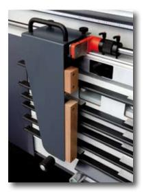
The robust flip stop (with fine adjustment) on a 30 mm solid shaft guidance, can be equipped with a square stop-extension.
